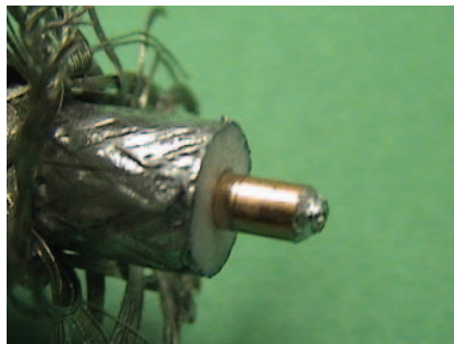
Prepped with a sharp knife
