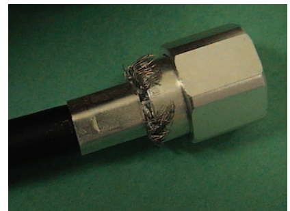
Exposed braid and double crimp (worst case)
