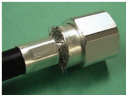
Crimp pushed back from connector due to excess braid
