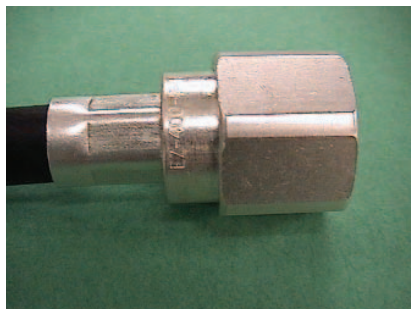
Proper crimping of ferrule
