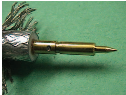
Pin too close to core with slight melting of core
