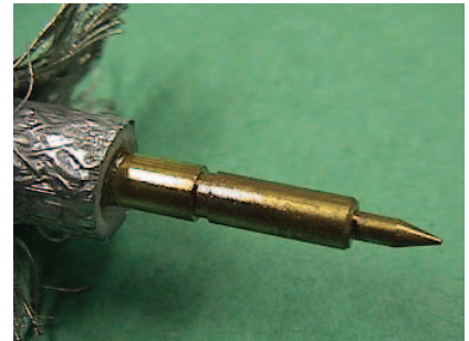
Pin pushed into the core with increased melting of core
