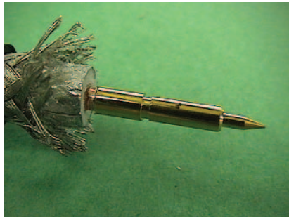
Proper soldering of pin
