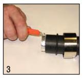
Step 3: Locate the inner drain wire (opposite the outer drain and under clear inner jacket). Slit the inner clear poly along the inner drain wire and pull back towards the jacket. Both drain wire will be exposed.
