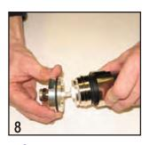
Step 9: Push in the connector inner conductor into the hollow copper tube inner cable conductor. Push on the connector head and attach to the backnut.
