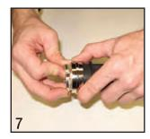
Step 8: Slide on the gland washer over both drain wires. The gland washer will seat against the outer jacket. Push back each drain and push on the slotted collar over the tape. NOTE: The gland washer and collar are angled for proper fit. Both drain wires will be clamped between the gland washer and collar.
