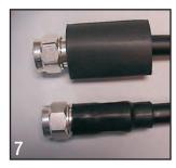
Step 5: Slide the connector over the end of the core and push it up to the end of the jacket. Rotate the connection back and forth in a clockwise-counter clockwise motion in reference to the axis of the cable until the back of the connector works its way under the end of the jacket. Now push the connector onto the cable with some back and forth motion until it stops.
