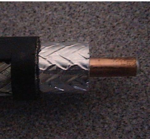
wrapped aluminum composite tape that is covered by a high-coverage, tinned copper round-wire braid. This cable is designed for applications that will see continued flexing, such as the portable point-to-point microwave antenna setups used by television news-gathering teams.
