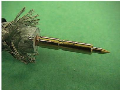
*Proper soldering of pin*
